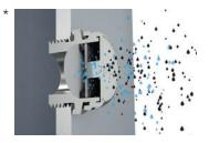
A quick balancing of pressure prevents the build-up of condensation water
